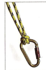
Fig. 17 Karabiner with a larksfoot to rope to maintain alignment
