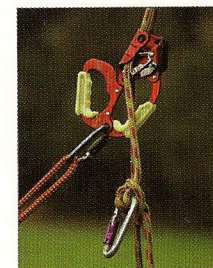
Fig. 81 Aerial rescue from a footlock line – back-up knot below friction hitch or ascenders
