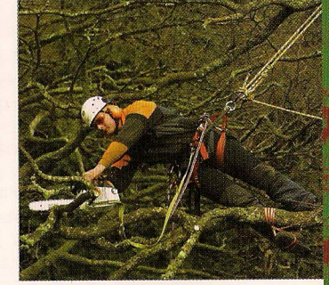
Fig. 71 Use of chainsaw, work position cutting away from body and ropes
