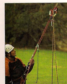
Fig. 80 Using the footlock line as an anchor point for the aerial rescue
