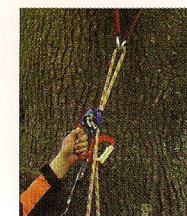
Fig. 53 Using friction saver with the footlock line to avoid 'V' in the rope caused by a branch
