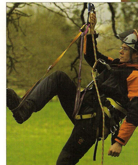
Fig. 57 Single rope technique attachment of ascenders
