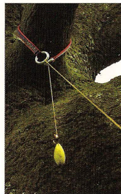
Fig. 30 Installation of friction saver from ground
