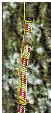
Fig. 49 Attaching throwline to climbing line with a clove hitch and half hitches for pulling rope through a friction saver
