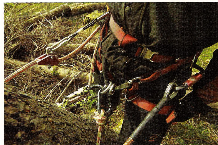
Fig. 68 Working from climbing irons – steel-cored flip-line backed up by climbing system
