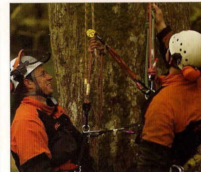
Fig. 75 Aerial rescue method A – use of a pulley above the casualty's friction hitch
