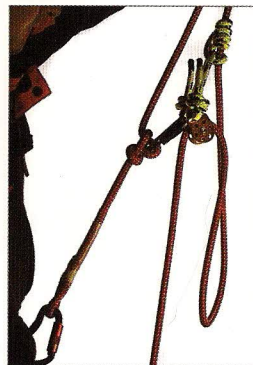
Fig. 25 Micro-pulley used to haul chainsaw in to tree
