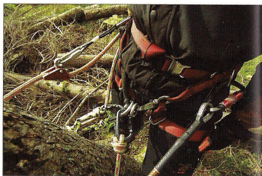
Fig. 58 Steel-cored flip-line with a 'soft link' when using a mechanical adjuster
