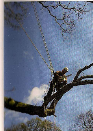
Fig. 72 Use of chainsaw, cutting away from the climber's ropes using a load bearing supplementary anchor
