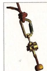
Fig. 16 Karabiner used with a clip/band to maintain alignment
